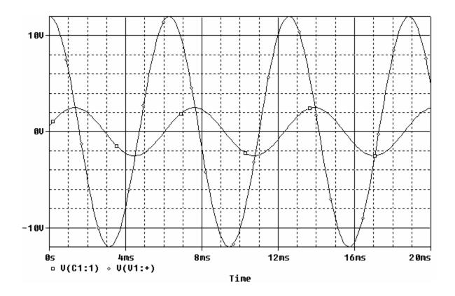
Some points on the input plot:  $v_i(0.00132) = 2.5 \text{ V} (\max v_i)$  and  $v_i (0.00446) = -2.5 \text{ V} (\min v_i)$ ;  $v_i (0) = 0.6048 \text{ V}$ .
