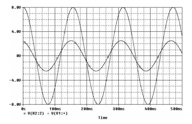
Some points on the input plot:  $v_i (0.0722) = -2.5 \text{ V} (\min v_i)$  and  $v_i (0.151) = 2.5 \text{ V} (\max v_i)$ ;  $v_i (0) = 2.43 \text{ V}$ .
